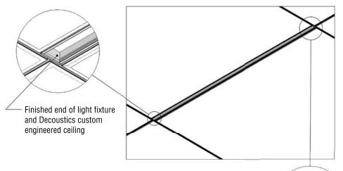
**LED Ceilencio Grid with Lighting Fixture Installed - Finished Ceiling Face** Image above shows ceiling utilizing the Ceilencio suspension system with the LED light fixture installed into the ceiling face. Note that the LED fixture is installed into the ceiling structure with a minimun 1/8" reveal around the perimeter of the fixture.
