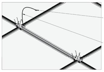
Electrical connector to be supplied attached to the light fixture by the lighting fixture supplier
