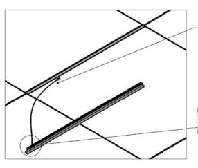
Power cable from the LED Ceilencio fixture. The power cord is fed through the wiring access hole in the grid rail into the plenum space above the ceiling.
