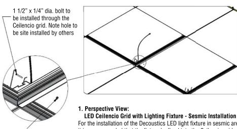
For the installation of the Decoustics LED light fixture in sesmic areas, it is recommended that the fixture be fixed into the Ceilencio grid rail. This can be very easily accomplished by drilling a hole, (by others) through the Ceilencio grid rail and LED light fixture and installing a 1 1/2" x 1/4" bolt. The bolt must be secured with a nut to lock the bolt into place.
