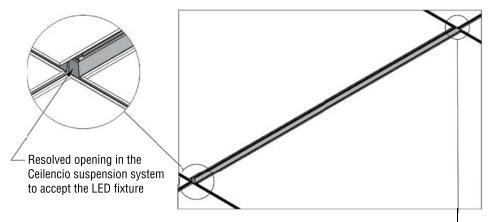
LED Ceilencio Grid Rail Opening in a Typical Ceilencio Ceiling Installation
