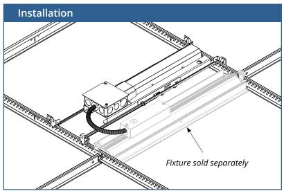
The battery backup kit is provided with a pair of adjustable T-BAR mounting brackets for simple installation in close proximity to the LED fixture (*sold separately*). They can be adjusted to fit over various typical grid spacing patterns (i.e 2x2) and also DESIGNFlex® grid layouts. Alternatively the kit can be surface mounted using the provided four mounting holes.
