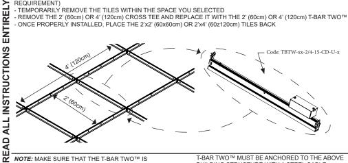
NOTE: MAKE SURE THAT THE T-BAR TWO™ IS POSITIONED TO ALLOW THE CORRECT PLACING OF THE CORRESPONDENT TILES
