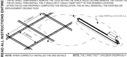
NOTE: WHEN CORRECTLY INSTALLED THE END DETAILS WILL ENSURE THE T-BAR TWO™ IS POSITIONED COR-RECTLY ALLOWING FOR THE CORRECT SPACING OF THE ARMSTRONG CEILING TILES
