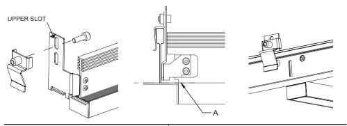
THE SLOTS ON THE MOUNTING BRACKET ARE DESIGNED TO ACCOMMODATE DIFFERENT **GRID HEIGHTS**
