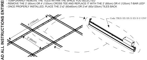
NOTE: MAKE SURE THAT THE T-BAR LED® IS POSITIONED TO ALLOW THE CORRECT PLACING OF THE CORRESPONDENT TILES
