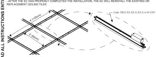
NOTE: WHEN CORRECTLY INSTALLED THE END DETAILS WILL ENSURE THE T-BAR LED® IS POSITIONED CORRECTLY ALLOWING FOR THE CORRECT SPACING OF THE ARMSTRONG CEILING TILES
