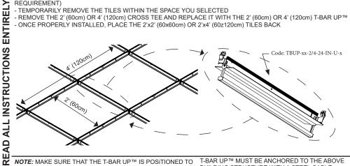
**NOTE:** MAKE SURE THAT THE T-BAR UP™ IS POSITIONED TO ALLOW THE CORRECT PLACING OF THE CORRESPONDENT **TILES**
