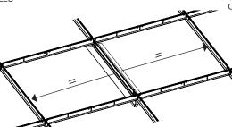
T-BAR UP™ MUST BE ANCHORED TO THE ABOVE BUILDING STRUCTURE WITH A STEEL CABLE USING THE CENTER HOLE. (STEEL CABLE BY OTHERS)
