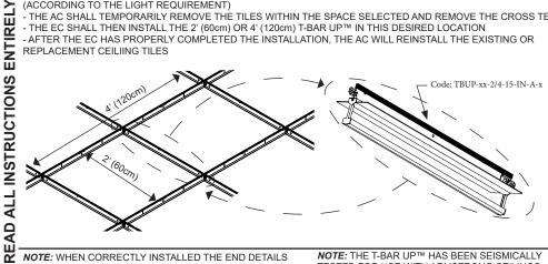
NOTE: WHEN CORRECTLY INSTALLED THE END DETAILS WILL ENSURE THE T-BAR UP™ IS POSITIONED COR-RECTLY ALLOWING FOR THE CORRECT SPACING OF THE ARMSTRONG CEILING TILES
