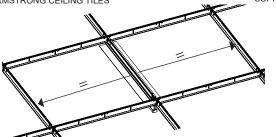
NOTE: THE T-BAR UP™ HAS BEEN SEISMICALLY TESTED FOR USE WITH ARMSTRONG CEILINGS AND DOES NOT NEED TO BE INDEPENDENTLY SUPPORTED
