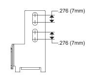
ONCE THE PRODUCT IS POSITIONED TIGHTEN THE SCREW ON EACH END
