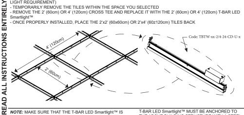
NOTE: MAKE SURE THAT THE T-BAR LED Smartlight™ IS POSITIONED TO ALLOW THE CORRECT PLACING OF THE CORRESPONDENT TILES
