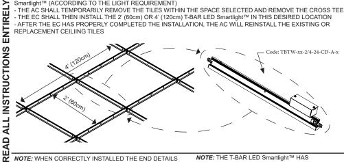
NOTE: WHEN CORRECTLY INSTALLED THE END DETAILS WILL ENSURE THE T-BAR LED Smartlight™ IS POSITIONED CORRECTLY ALLOWING FOR THE CORRECT SPACING OF THE ARMSTRONG CEILING TILES
