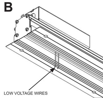
**⚠** IMPORTANT: VERIFY LOW VOLTAGE WIRES ARE PULLED INTO SORELLA™ HOUSING FROM JUNCTION BOX, BEFORE PROCEEDING WITH THE INSTALLATION OF THE SORELLA™ HOUSING.
