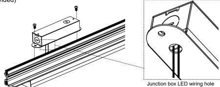
5. Open the cover of the junction box, and first make the low voltage connections from the driver to the LED board using the provided lever connectors, according to the following wiring chart:
