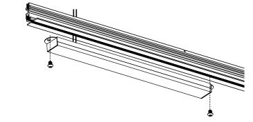
4. Using the provided junction box, pass the wires thru the hole in the bottom of the junction box (into the driver compartment). Mount the junction box into position on the upper threaded boss channel using 1/4-20 x 1/2" screws (provided)
