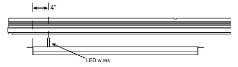
2. Using a 1/4" drill bit, drill a hole through the Dynamax™ grid in either one of the locations below to allow for the LED wires to pass through the Dynamax™ grid and into the wiring hole in the bottom of the junction box.
