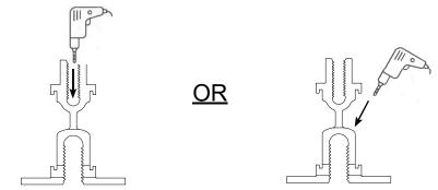
3. Holding the fixture into position, pass the LED wires thru the drilled hole in the lower threaded boss channel and mount the fixture into place with the end brackets using  $3/8-16 \times 1/2$ " screws (provided)
