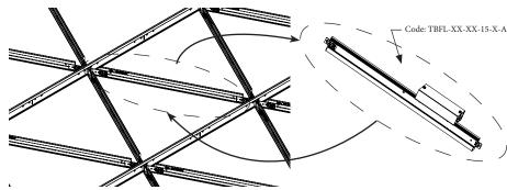
NOTE: WHEN CORRECTLY INSTALLED THE END DETAILS WILL ENSURE THE T-BAR FLEX IS POSITIONED CORRECTLY ALLOWING FOR THE CORRECT SPACING OF THE ARMSTRONG CEILING TILES
