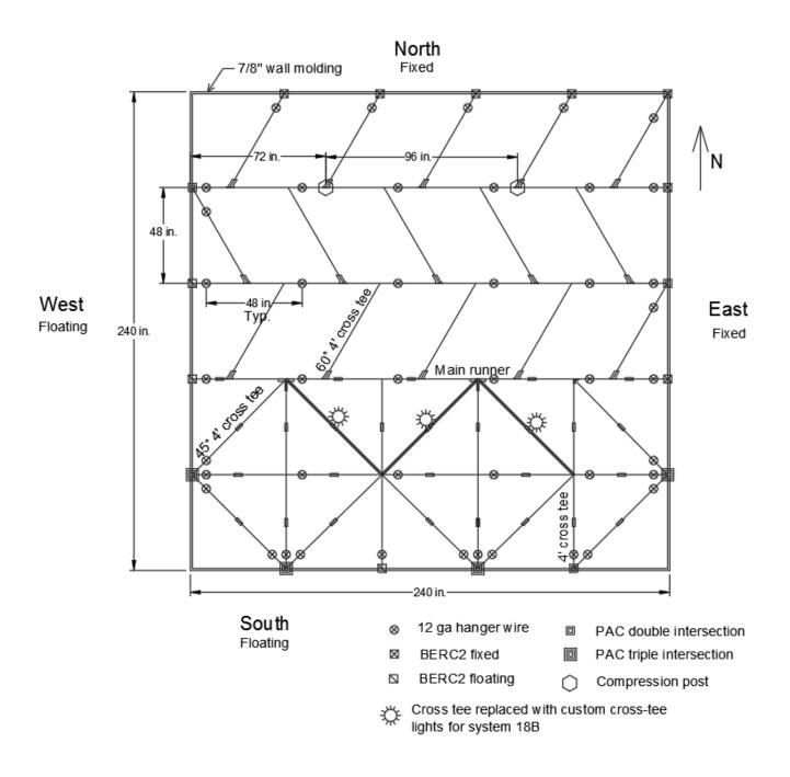
Figure 1: Layout of grid and panels for ceiling systems 18 and 18B
