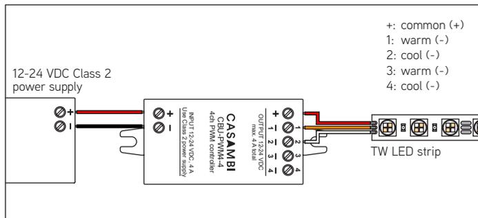
**Wiring diagram, 1-4 separate channels**
