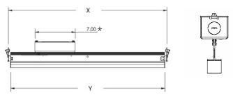
\* Junction box length may be different for options other than standard universal input 0-10V dimming driver or other controls options, refer to the controls guides on website for more information.
