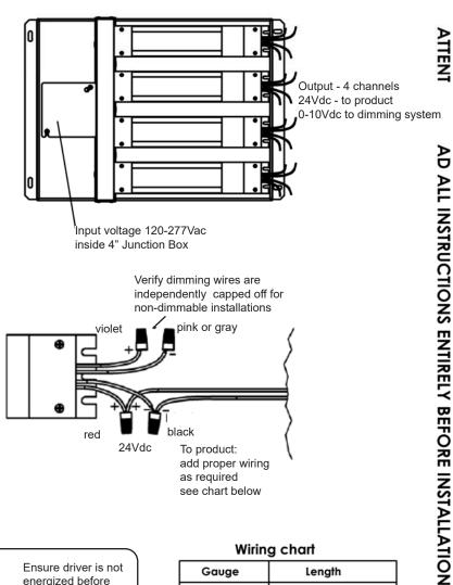
Verify dimming wires are independently capped off for non-dimmable installations
