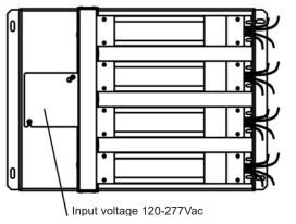
Output - 4 channels 24Vdc - to product 0-10Vdc to dimming system
