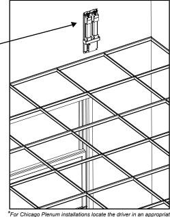
\*For Chicago Plenum installations locate the driver in an appropriate enclosure (by others) or in a non-Chicago Plenum rated area.
