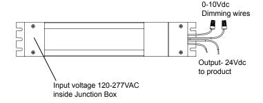
To dimming system: add proper wiring as required
